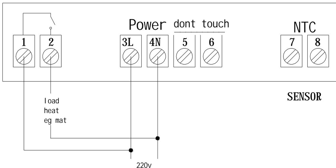
Terminals 1 and 2: Normally opened contact of relay
