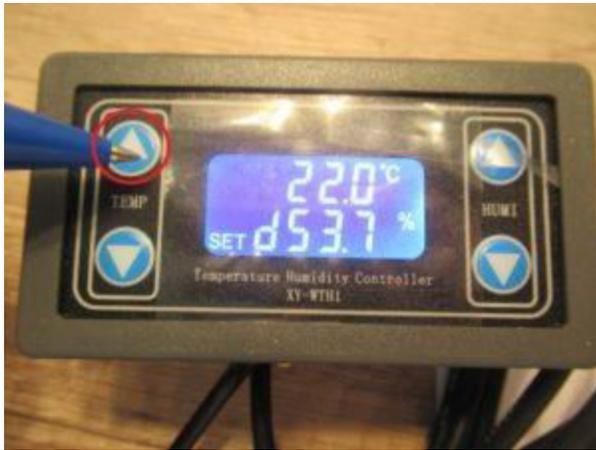
2. In the running interface, Long Press **TM-** key more than 3 seconds, into the stop temperature settings interface, can be modified by **TM+** **TM-** key, to be modified after the parameters, waiting for 6s automatic exit and save;
