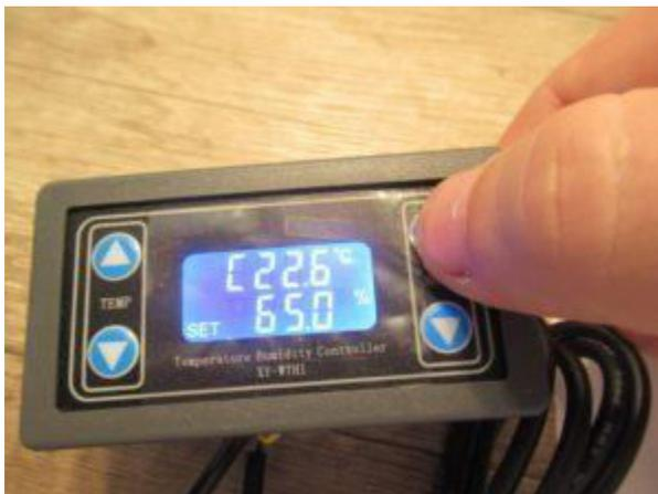
2. In the running interface, Long Press 'RH-' key more than 3 seconds, into the stop humidity settings interface, can be modified by RH+ RH- key, to be modified after the parameters, waiting for 6s automatic exit and save.
