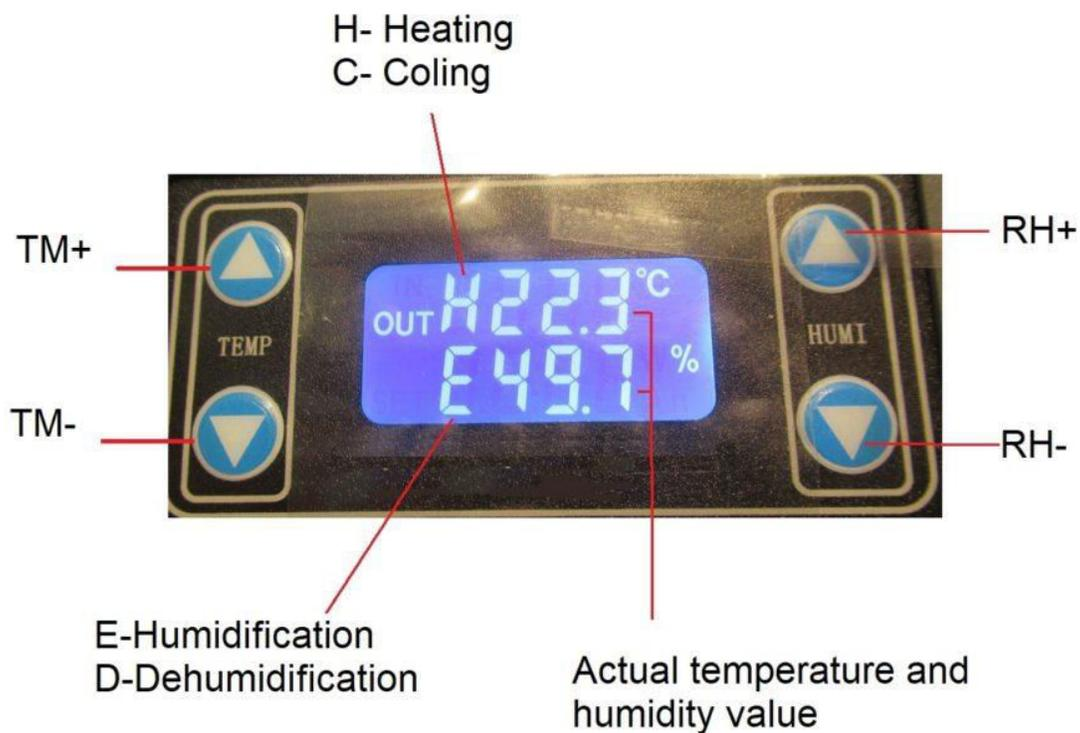
How to set the temperature for heating or cooling:
